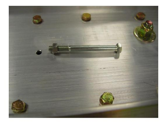
THERE IS A LOCK BOLT PROVISION AS WELL. PLACING A 1/4" x 3.5" BOLT IN THE HOLE WILL LOCK THE INTERNAL MECHANISM SO THE GATE SAVER CANNOT MOVE OUT OF THE CENTER POSITION. THIS PROVISION IS INTENDED FOR SEVERE STORMS LIKE A HURRICANE WHERE THE WINDS WILL BE MUCH HIGHER THAN TYPICAL AND THE POSSIBILITY OF BEING BLOWN OUT OF THE WIND BRACKET IS HIGH.
