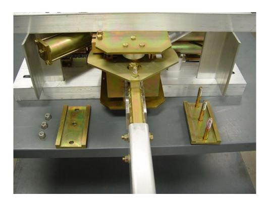
FOR SERVICE THE ARM CAN BE SWUNG OUT OF THE WAY. REMOVE THE 3 BOLTS HOLDING THE ARM SIDE PLATES. LOCK THE MECH IN THE DOWN POSITION. AS SHOWN ABOVE THE ARM IS AT CENTER, BUT THE ARM WILL SWING EITHER DIRECTION 90 DEGREES.
