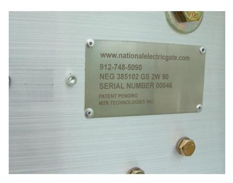
ALL 90 DEGREE 2WAY GATE SAVERS ARE UNIQUELY IDENTIFIED BY SERIAL NUMBER. THE ID PLATE IS LOCATED SO IT IS READILY VISIBLE WHEN THE MECH IS UP.
